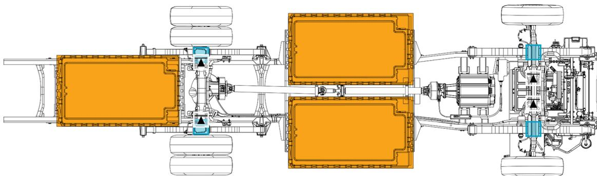
High Voltage Component    Jacking Points    Lifting Points
